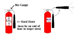
**Carbon dioxide** extinguishers are generally used in areas of sensitive electrical or electronic equipment since it is gas and leaves no residue that damages the equipment. Carbon dioxide functions by removing or displacing the oxygen in a fire. It is a non-flammable gas, extremely cold.
