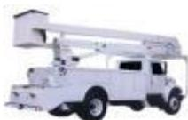
**Vehicle mounted bucket lifts** - Are usually attached to a vehicle and used to repair utility lines.
