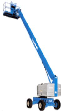
**Extensible or telescoping boom lifts** - Are aerial devices with an extensible or telescopic boom. They are designed to reach vertically or horizontally.
